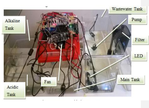
Figure 2.0. Hardware components interfaced with LabVIEW
